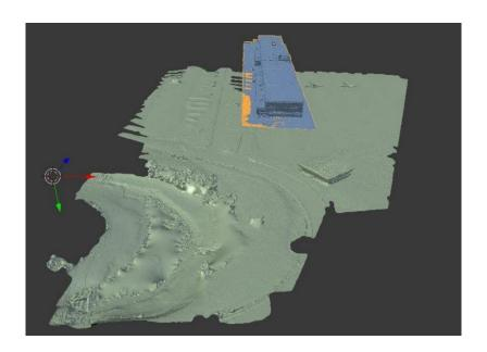
Figure 8. Three-dimensional model of hangar and surrounding terrain developed in Pix4D using imagery captured by the sUAS.
