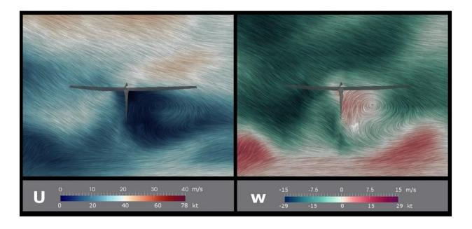
Figure 12. Vertical cross-section visualization of wind simulation results for a discrete time showing horizontal ("U") and vertical ("w") wind magnitudes in area of the accident airplane's elevators.
