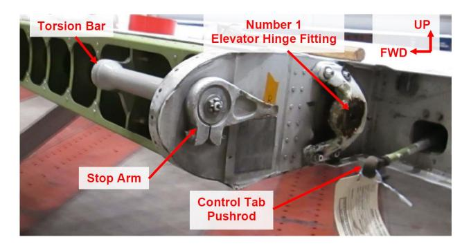
Figure 13. Elevator stop arm and torsion bar assembly.
