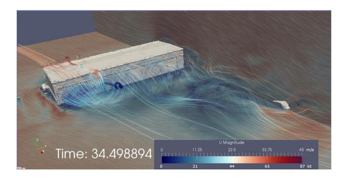
Figure 11. Three-dimensional visualization of wind simulation results for a discrete time showing turbulence generated downwind of the hangar. Note: Accident airplane's elevators can be seen on lower right side of image.
